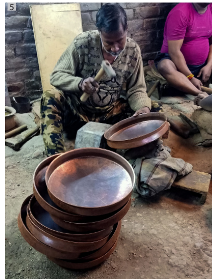
The molded forms beaten further into desired forms for utensils.
