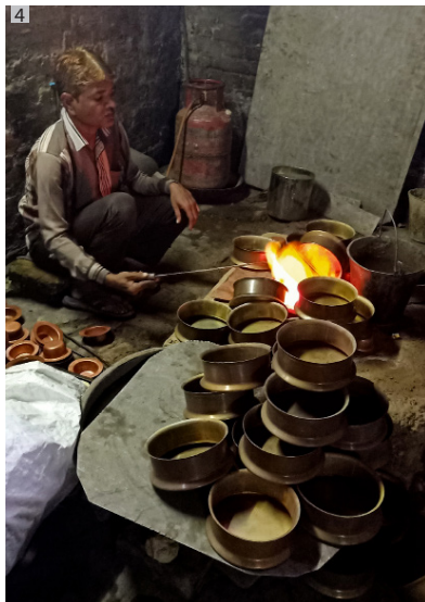
The press-molded vessels are heated to increase malleability.
