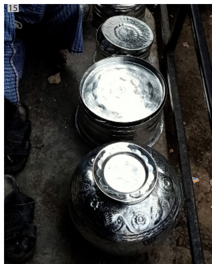
Kalai is also applied on the outer surface of vessels for ornamentation.
