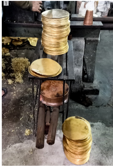
The metal sheets are cut into smaller sizes and desired forms.
