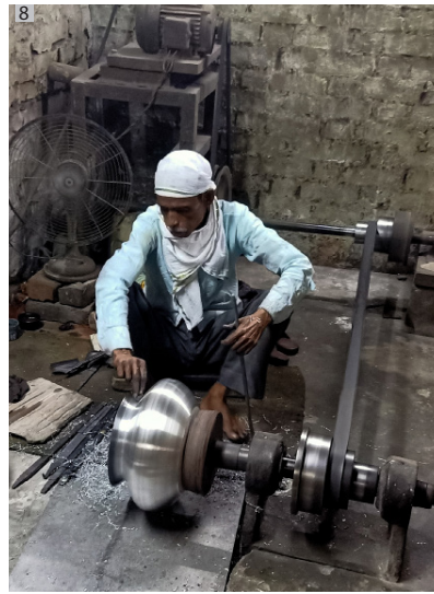
The vessels are then scraped to expose an even and shiny surface.
