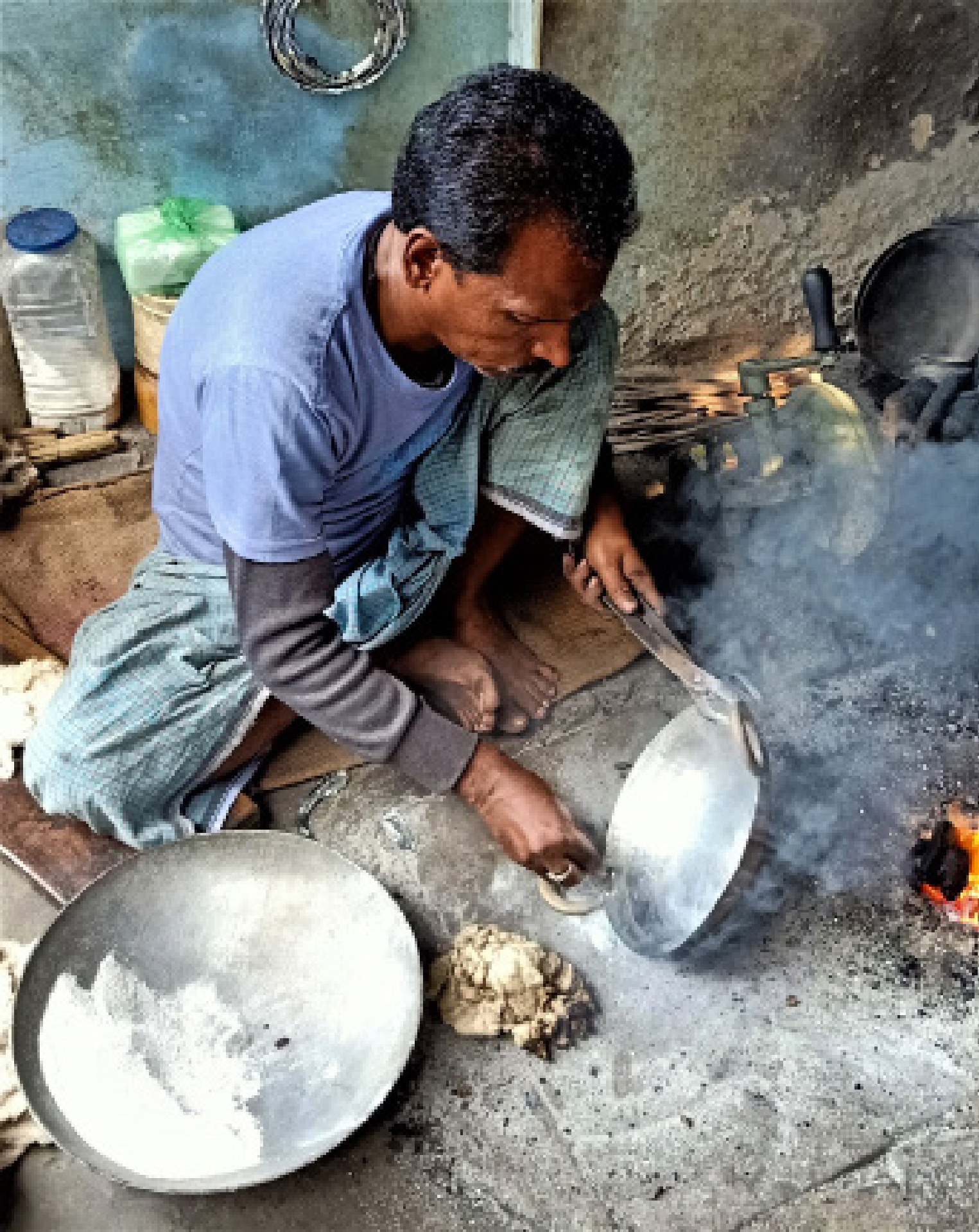
A rangaikar applying kalai on a finished vessel. Kalai makes a vessel foodsafe.
