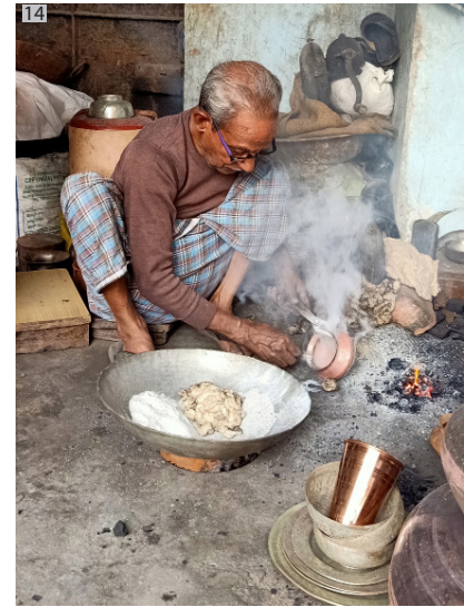
A craftsmen applying kalai on vessels inner surface to make it food safe.
