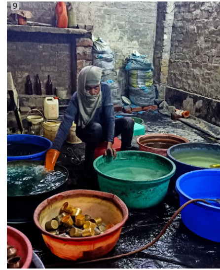
The vessels are washed very dilute HCl acid to remove the impurities.
