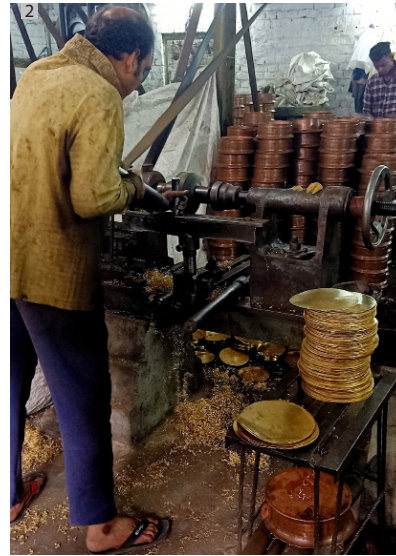
The sheets are then trimmed to remove the rough edges.
