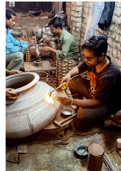
The bigger vessels, made in parts, are welded together.
