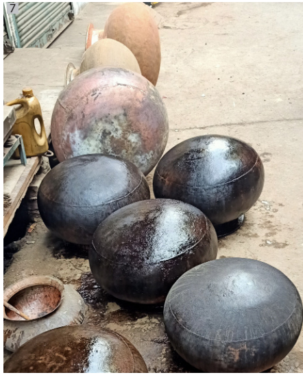
The vessels are covered with HCl acid to remove the outer layer.
